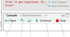
Step through Step into and Resume Ouit debug code one line out of functions execution mode
